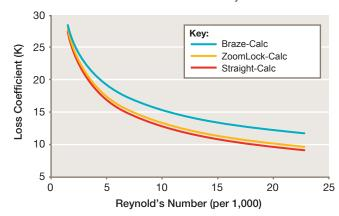
3/4" ACR Tube Loss Coefficient vs. Reynolds Number
